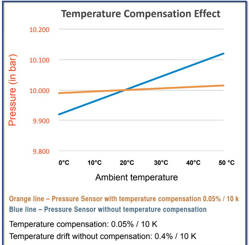
Manufacturers usually specify a temperature range the sensor should be used in. However, if there is no temperature compensation, the sensor's accuracy specification may not be met when the environment the sensor is used in — even if it is still within the temperature range specification, but significantly greater or less than ambient temperature.
