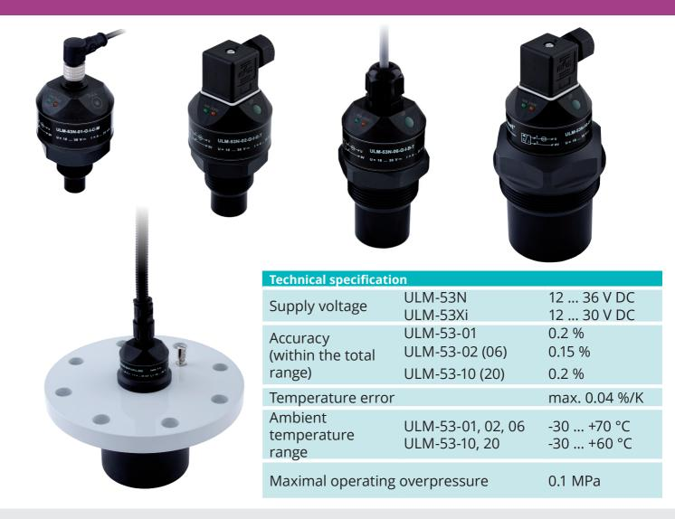
For continuous non-contact level measurement of various liquids, mashes and pasty materials in closed or open vessels, sumps, reservoirs etc.
